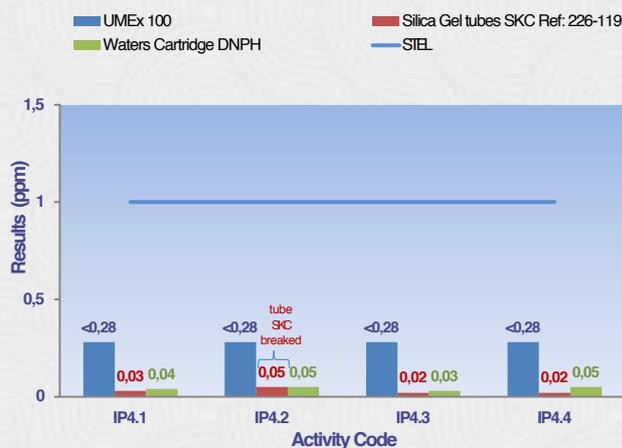
The same trend can be seen for the three activities carried out in Institut Pasteur's Laboratories and similar to SANOFI campaign: results of active technologies are always inferior to the passive technologies. It is remarkable that this time the batch expiration date was superior to the SANOFI's batch. This confirms the necessity of minimizing the time of storage before using the sampler.
