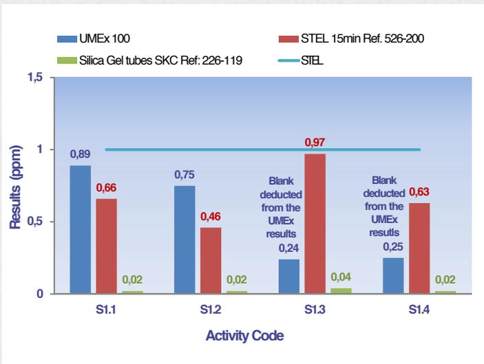
For the activity 1 (Figure 3) three samplers of short duration have been used: UMEEx100, STEL 15 and the tubes. The activity was repeated four times.
