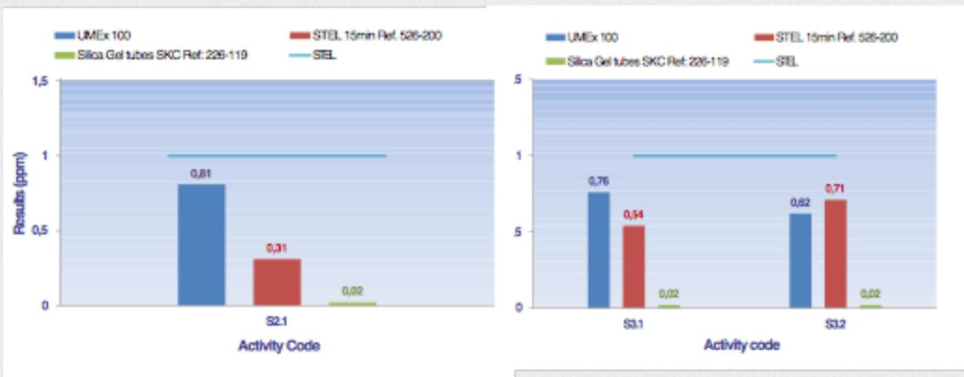
As can be noted in activities carried out at SANOFI (Figure 3 to 5) the tendency is similar: actives samplers' results (Silica gel tubes) are inferior to diffusional samplers' results (STEL 15 and UMEEx100). Results obtained with the tubes show a great repetitively. Regarding the UMEEx sampler it is necessary to take into account that two types of blanks were used:
