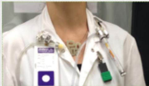
**Figure 2.** Samplers Fixation to the operator's blouse
